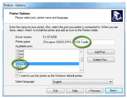
Uncheck any additional install options in the next dialog and select Finish. Close the Zebra Setup Utilities. In the Devices and Printers window right-click on the new driver entry and select 'Printer properties'.
