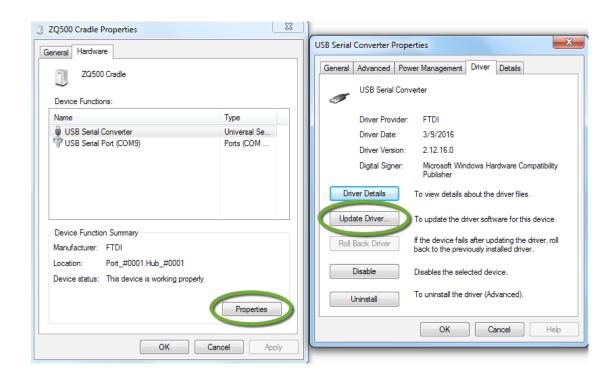
Once the driver for the cradle has been installed or updated, make sure the printer is turned on and run the Zebra Setup Utilities. If the System Prepare Wizard loads, select 'other computer ports', click Next, and then Install Printer. If the wizard does not run, then select 'Install Printer' from the main application window. Install the CPCL ZDesigner driver for your model printer.
