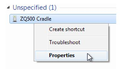
Install or update the driver for <u>both</u> the USB Serial Converter and the USB Serial Port. Reference the driver from the folder into which you download it earlier. Note new serial COM Port #.
