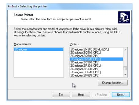
Select the virtual com port that was generated by the FTDI cradle driver (COM9: in this example). It is recommended that you modify the printer name for the driver so that it will be easy to see that this port is for the ZQ500 cradle.
